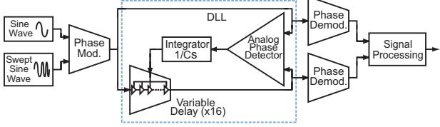
Fig. 4: Simplified functional model of first order analog DLL.
