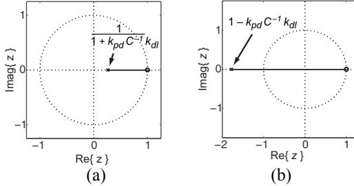
Fig. 9: Root-locus plot of first order charge-pump DLL using (a) proposed model and (b) the model from [2].
