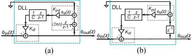
Fig. 8: Simplified z-domain model of the feedback loop in a first order charge-pump DLL: (a) proposed (b) model from [2].
