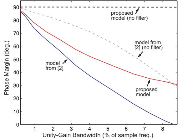
Fig. 11: Phase margin as a function of unity-gain bandwidth.
