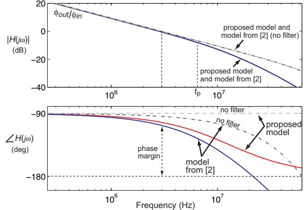
Fig. 10: Open-loop frequency response of first and second order charge-pump DLL from [2], with and without loop filter.
