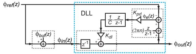
Fig. 7: Simplified z-domain model of first order charge-pump DLL.
