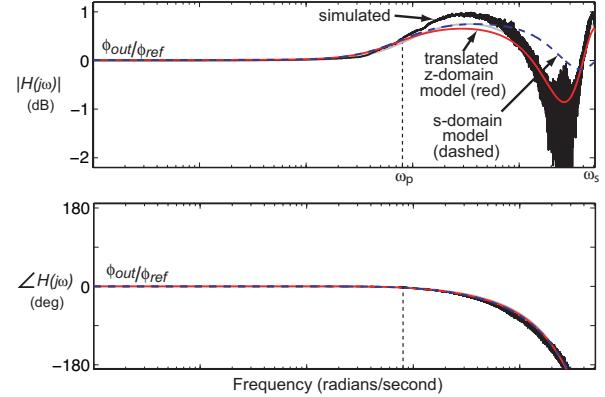
Fig. 6: Frequency response of a first order charge-pump DLL.
