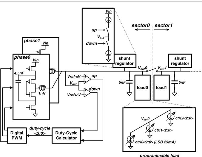
Figure 15.3.2: Block diagram of 3-level converter with slow digital feedback control and fast shunt regulation.
