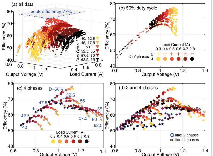
Figure 15.3.4: Measured conversion efficiency.
