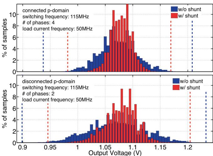
Figure 15.3.5: Histogram of measured voltage noise with and without shunt regulator for connected and disconnected power domains of two sectors.
