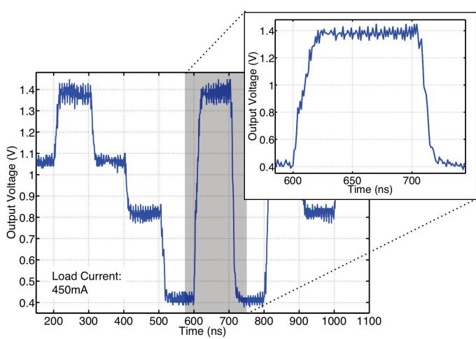
Figure 15.3.3: Measured snapshot of fast dynamic voltage scaling. Voltage scales from 1.4V to 0.4V and vice versa in 15-20ns.
