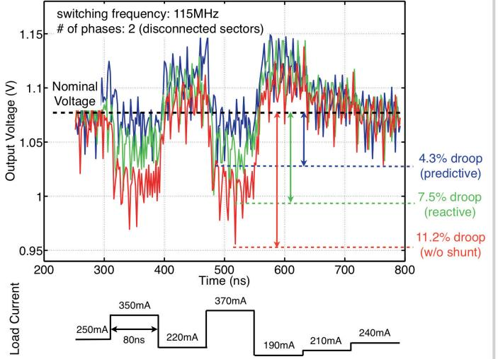
Figure 15.3.6: Comparison of measured on-die voltage noise without shunt regulator, with reactive shunt, and with predictive shunt.
