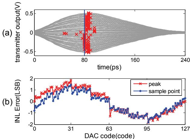
Fig. 4. Effects of within-die mismatch and DAC nonlinearity on pulse1 at 12.5-Gbps: (a) deviations in pulse peak position and (b) 7-bit DAC INL error.
