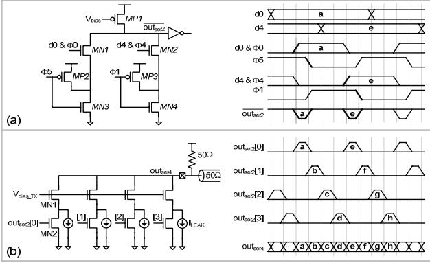
Fig. 2. Two-stage 8:1 serializer schematics and timing diagrams: (a) 2:1 multiplexer and (b) 4:1 multiplexer + current DAC.
