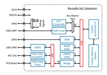
Fig. 2. Reusable SoC subsystem, extended with a custom IP block.
