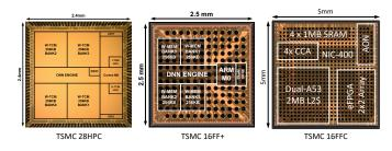
Fig. 1. Three recent chips [1], [2], [3] built using the CHPIKIT framework.
