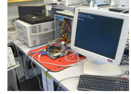
(d) Gathering oscilloscope data using an external system that connects over the network.
