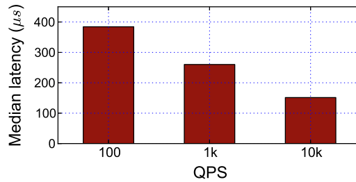
Figure 2.6: Round-trip latency degradation for a RPC transport layer for varying queries per second (QPS). Too aggressive sleep states (at low QPS) significantly degrade request latency.
