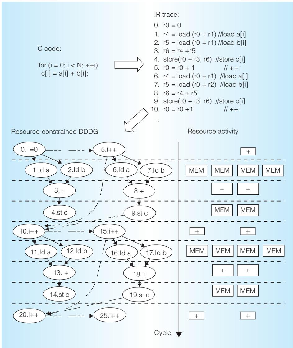
Figure 6. Different phases of Aladdin transformation illustrated with a microbenchmark: starting from a C code, to an intermediate representation (IR) trace, then a resource-constrained dynamic data dependence graph (DDDG), and finally a dynamic activity profile.
