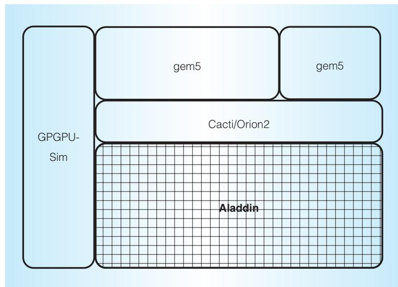
Figure 11. SoC simulation infrastructure with Aladdin. Aladdin can be integrated with other architectural simulators to model future heterogeneous SoCs.
