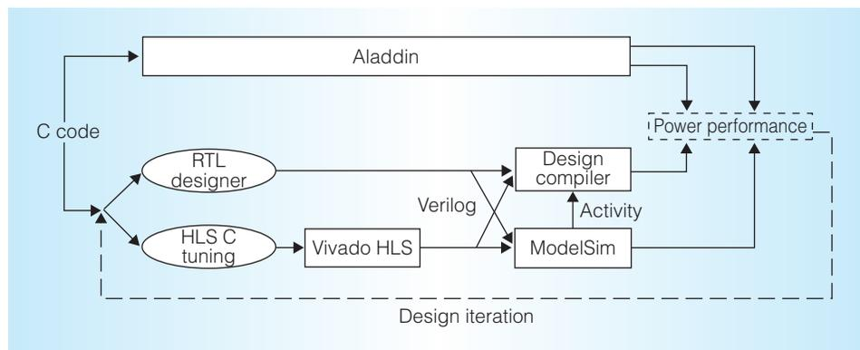
Figure 8. Aladdin validation flow. Aladdin’s estimates are compared against synthesized accelerators using commercial CAD tools.
