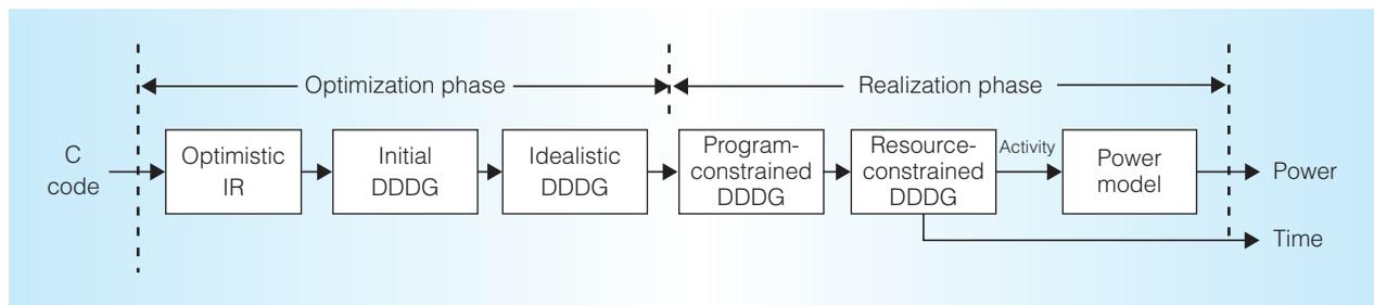
Figure 5. Overview of the Aladdin framework. Aladdin takes C code and passes it through an optimization phase and a realization phase to estimate an accelerator’s power and performance.
