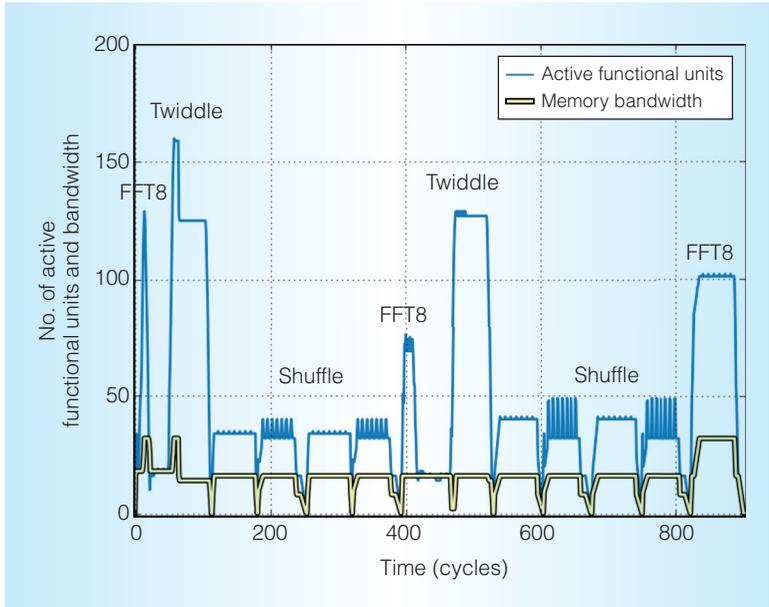
Figure 7. Realistic cycle-level functional units and memory activity of a fast Fourier transform (FFT) accelerator. This cycle-level activity is also an input to the power model to represent the dynamic activity of accelerators.
