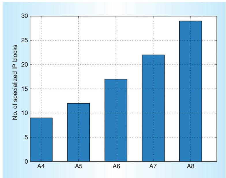
Figure 2. Number of specialized IP blocks across generations of Apple's SoCs. We see a consistent increase in the number of blocks.
