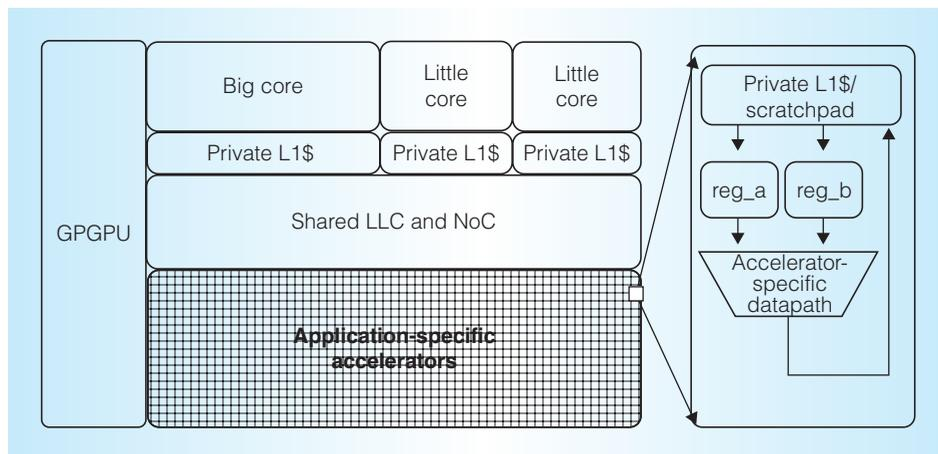
Figure 3. Future heterogeneous architecture will include a large number of customized accelerators. Large design space exploration is needed to design such architecture.
