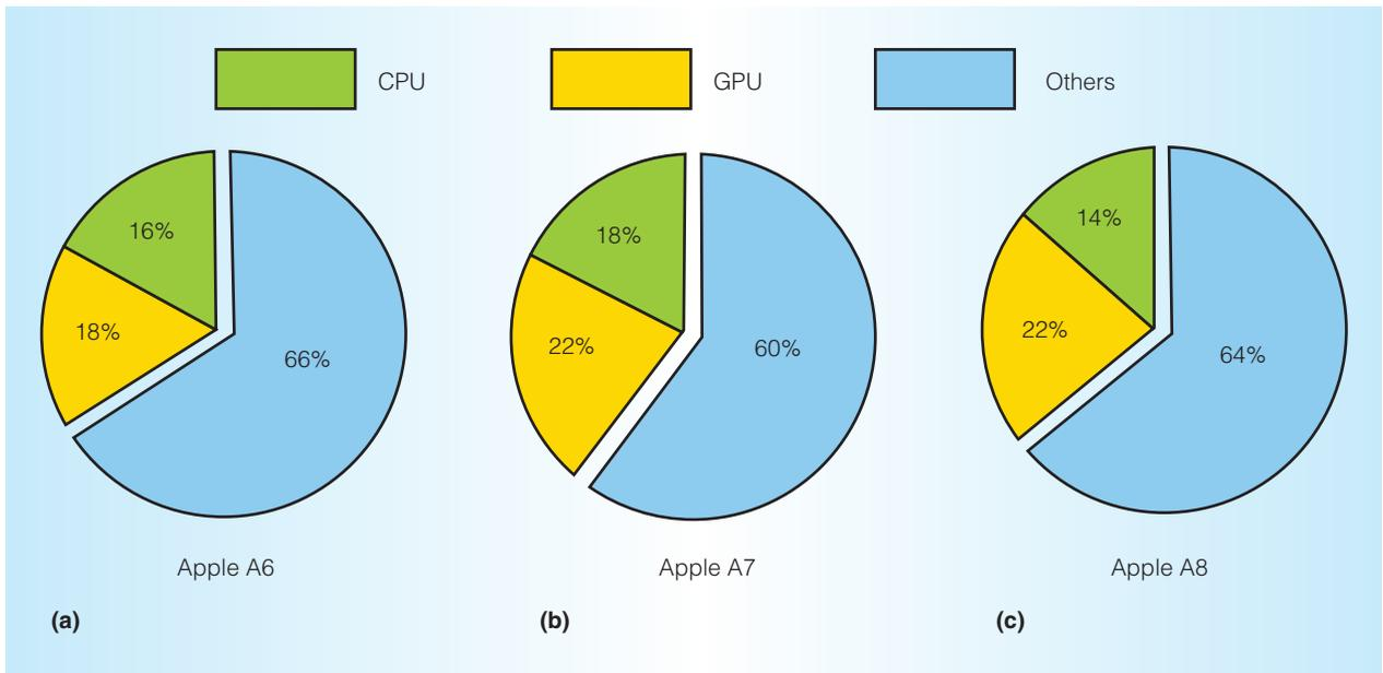
Figure 1. Die area breakdown of Apple's systems on chips (SoCs). (a) A6 (iPhone 5), (b) A7 (iPhone 5s), and (c) A8 (iPhone 6). More than half of the die area is dedicated to specialized IP blocks.
