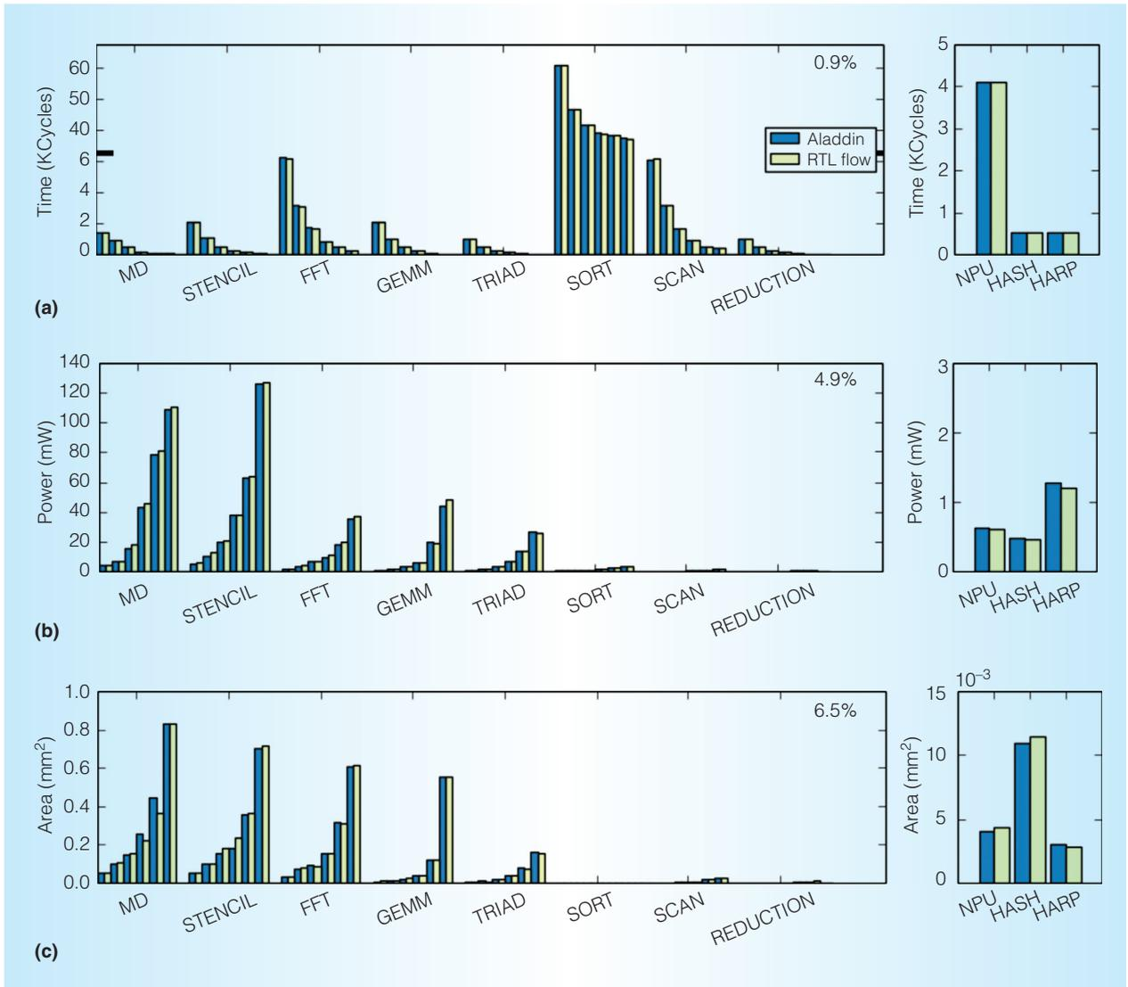
Figure 9. Aladdin validation results against RTL implementations. (a) Performance, (b) power, and (c) area validation. Aladdin accurately models performance, power, and area across various benchmarks.
