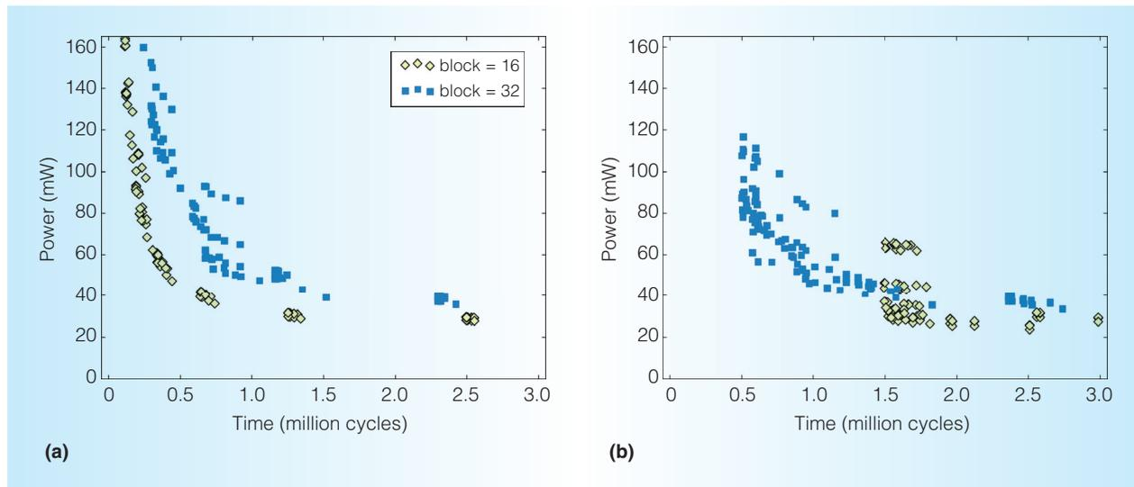
Figure 10. GEMM design space: (a) without contention and (b) with contention. A blocking factor of 16 outperforms a blocking factor of 32 when no memory contention presents, but the opposite occurs when there is memory contention.
