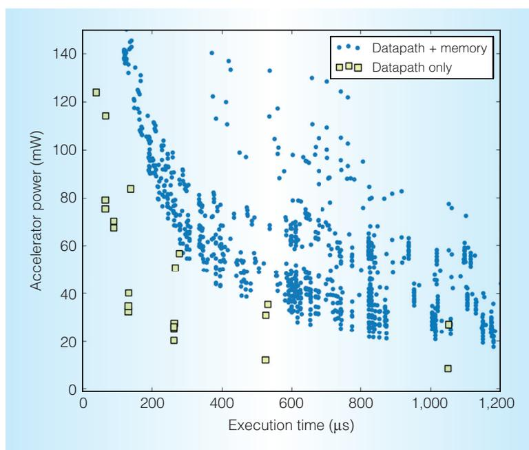
Figure 4. GEMM design space. A large design space is overlooked if we ignore the memory parameters.
