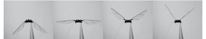
Fig. 6. High-speed video frames of HMF wings flapping at 100Hz (asymmetry is due to manufacturing imperfections).
