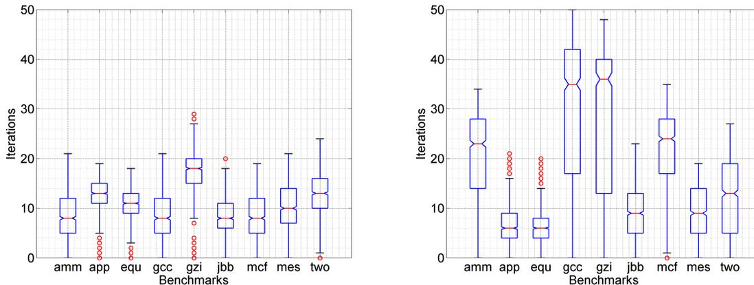
**Figure 10.** Distribution of gradient ascent convergence times for 1,000 trials performance (a) and efficiency (b).
