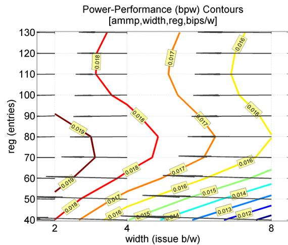
**Figure 4.** *Ampm* power-performance contours for depth and width (a), register file and width (b).
