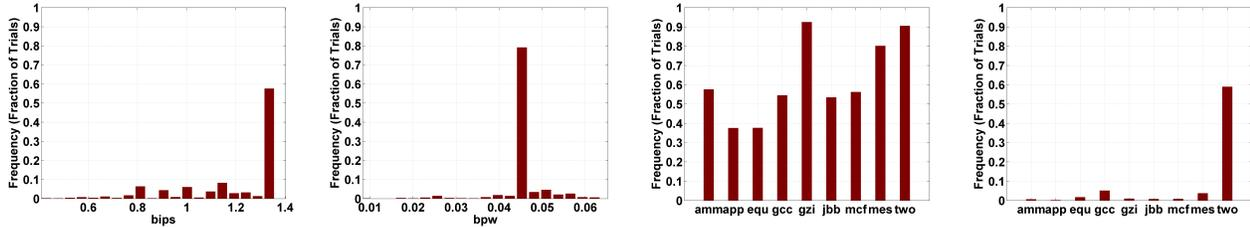
**Figure 9.** Histogram of *ammp* gradient ascent results for performance (a), efficiency (b). Percentage of trials with performance (c), efficiency (d) in the optimal bin.
