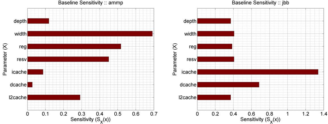
**Figure 2.** Sensitivity computed at a POWER4-like design for *ammp* (a) and *jbb* (b).
