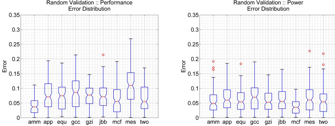
**Figure 1.** Distribution of performance (a) and power (b) modeling errors for 100 random validation designs.
