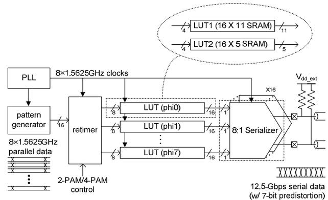
Fig. 1. Overall transmitter block diagram
