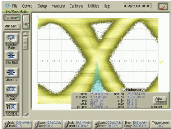
Fig. 7. Histogram of zero crossings for mean and rms jitter measurement.
