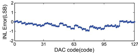
Fig. 5. Effects of DAC current mismatch and nonlinearity on pulse1 at low frequency (~5 Gbps).
