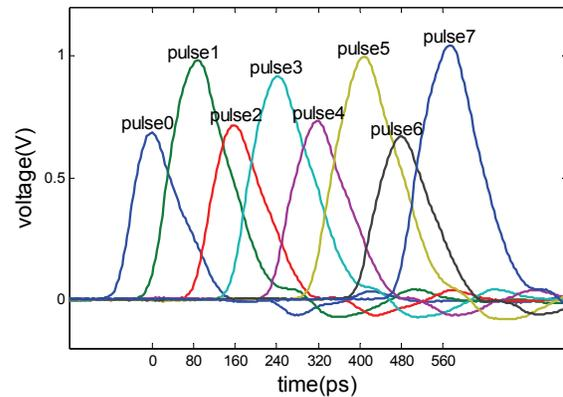
Fig. 3. Transmitter pulse responses through 8 interleaved paths.
