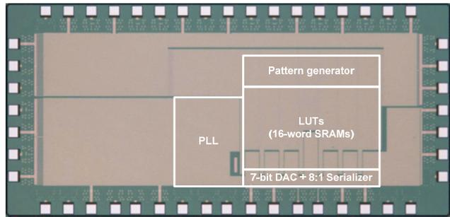
Fig. 9. Die photo and overlay of basic blocks.
