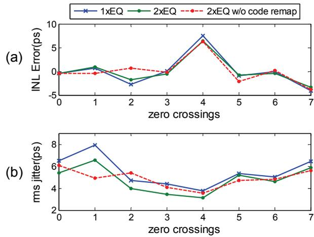
Fig. 8. Data transition point measurements: (a) mean INL error, (b) rms jitter.
