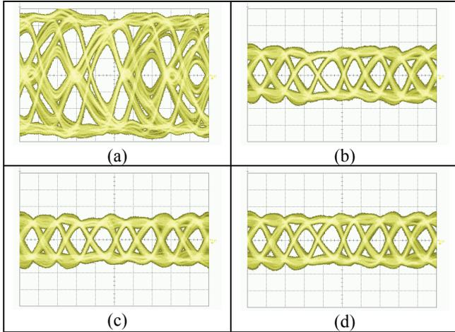
Fig. 6. Eye diagrams of transmitter at 12.5-Gbps: (a) without equalization, (b) with 2xEQ before LUT code remapping, (c) with 1xEQ, and (d) with 2xEQ after LUT code remapping.
